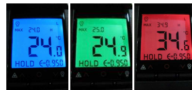
Temperature Display changes color upon Hi/Lo setpoint.
