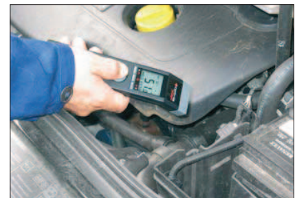
Temperature Display changes color upon Hi/Lo setpoint.
